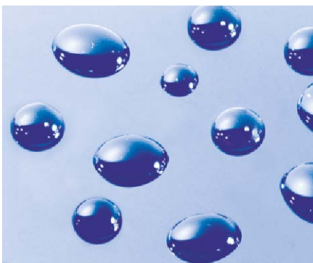
Fig. C1.65 Self-cleaning glass coating with silicon-chemical compounds that allow for water to drip off easily
