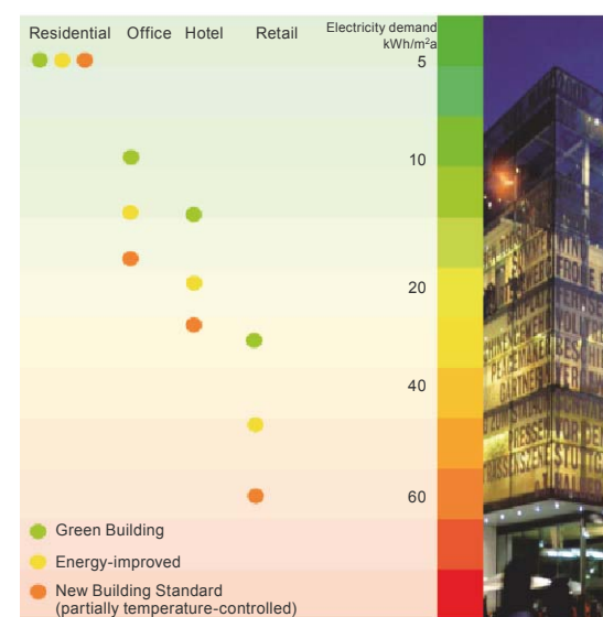
Fig. B2.15 Parameters for Electricity Demand for artificial lighting in Central Europe for different utilizations
