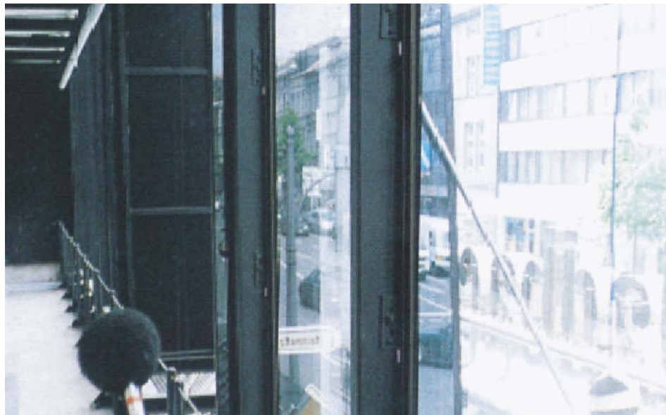
Fig. C3.9 Sound Measurement in the interim façade space and outside for a double-skin façade
