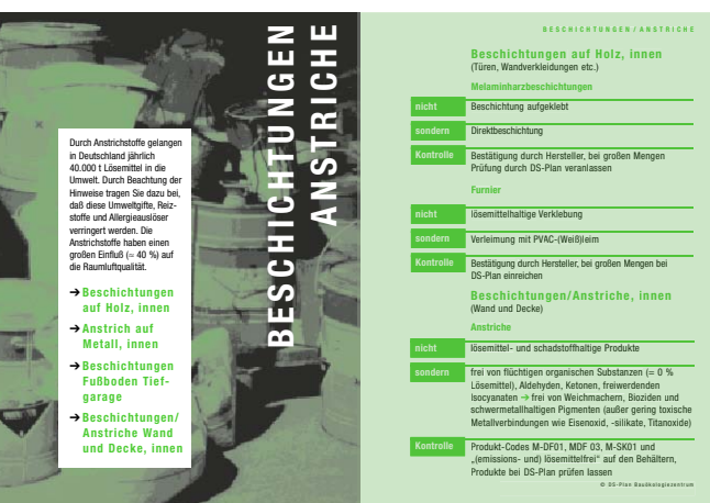
Fig. C1.50 Excerpt from a D&S Advanced Building Technologies handbook for prime contractors titled »Building Ecology«. Here: Requirements for coatings and paints
