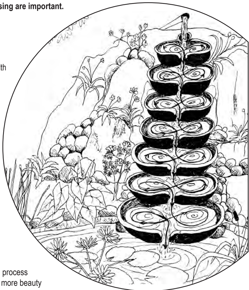
A Future Technology for East Timor: Clay Flow Forms that help clean and add oxygen to water.
