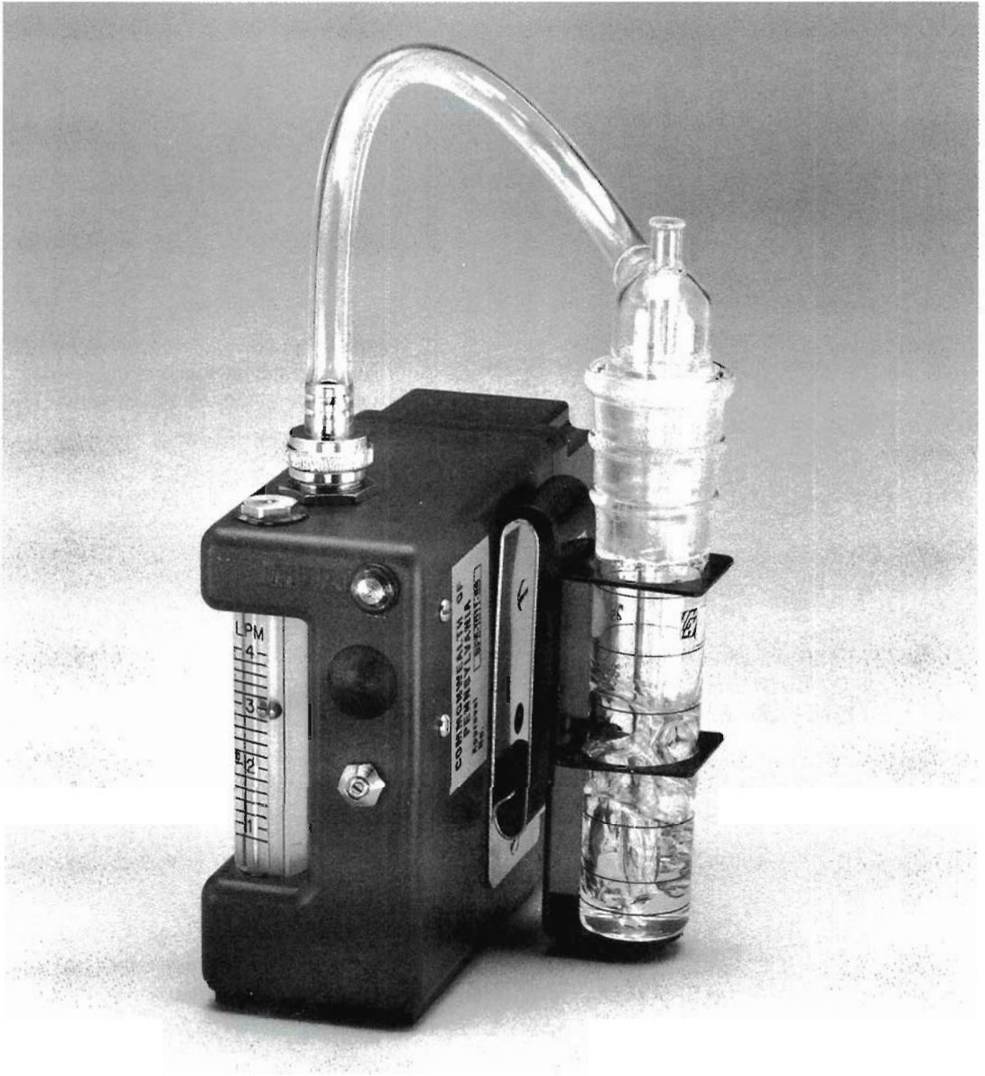
Figure 11-11. Pump with impinger (container) used for collecting and ascertaining viable particles present in air samples. Courtesy Mine Safety Appliances Co.
