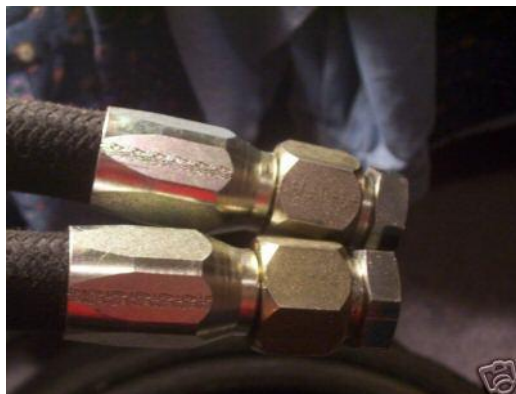
Hose with Aeroquip fittings
