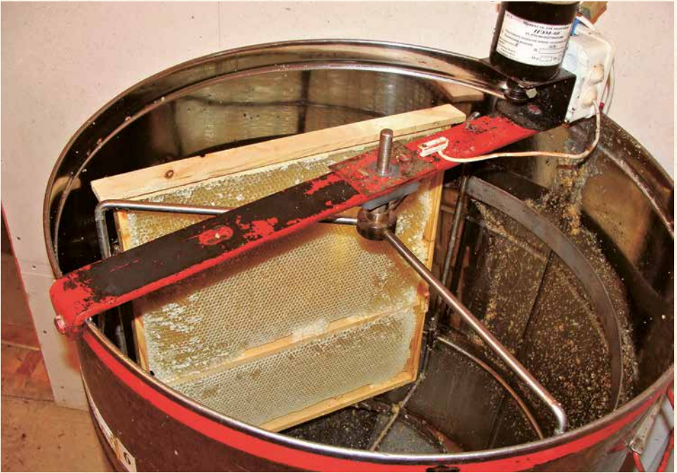
PHOTO 49. Spinning frames in a centrifugal extractor removes honey without crushing the wax comb, which can then be reused.
