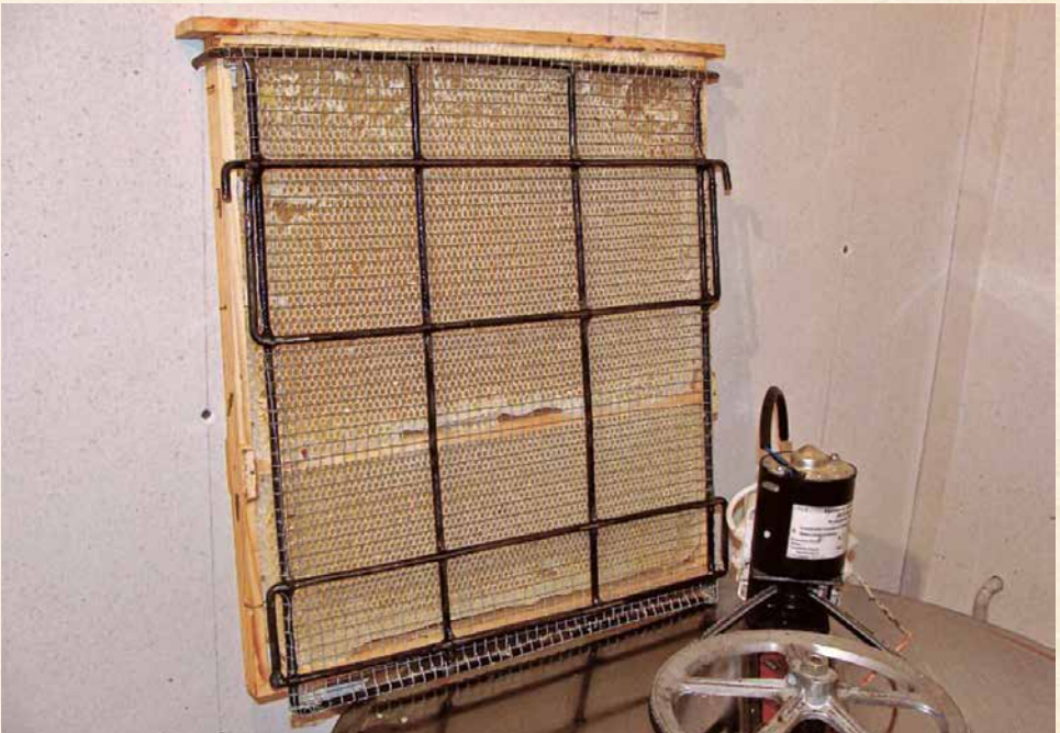
PHOTO 50. As long as your extractor is big enough, you can make a special insert to hold the extra-deep frames.
