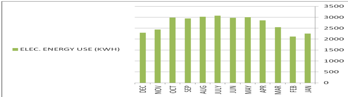
Figure 21: Monthly electric energy consumed by the passive energy system.
