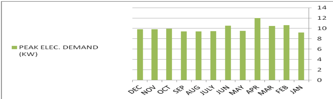
Figure 22: Monthly peak electric energy demand by the active energy system.
