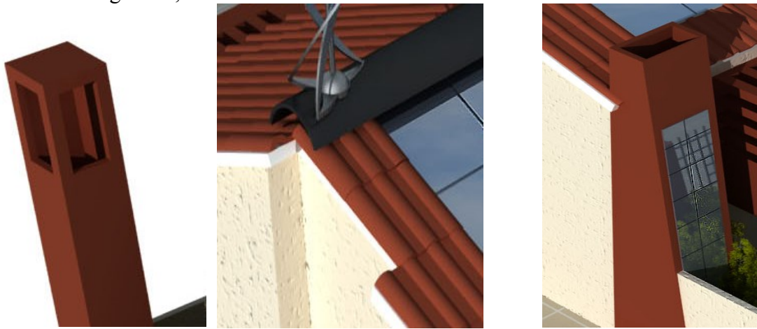
Figure 8: four cross opening wind catcher for the Suggested prototype house.
